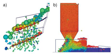
Fig. 1: Examples of granular material analysis: a) screening/separation; b) feeders, hoppers, storage facilities
