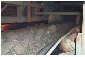
Fig. 11: Material on BC 401 conveyor belt from the new BC 400 chute
