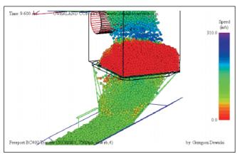
the chute to help to center load the receiving belt-conveyor. It looks like a very straightforward chute with the angle between the incoming and outgoing conveyor of 130.72°. The major problems that were reported by the mine site were as follows:
