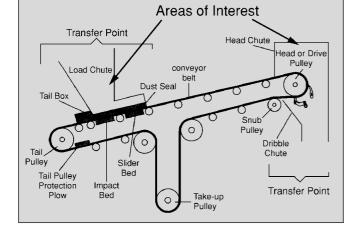
other loading equipment is heavily influence by conditions such as the capacity, size, vertical drop, characteristics of the material handled, speed and inclination of the belt and whether it is loaded at one or several locations. An ideal transfer point would be designed to take into account the following:
