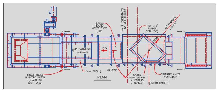
Fig. 10: Original geometry and overall chute layout
