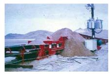
Fig. 4: Plugging and spillage
